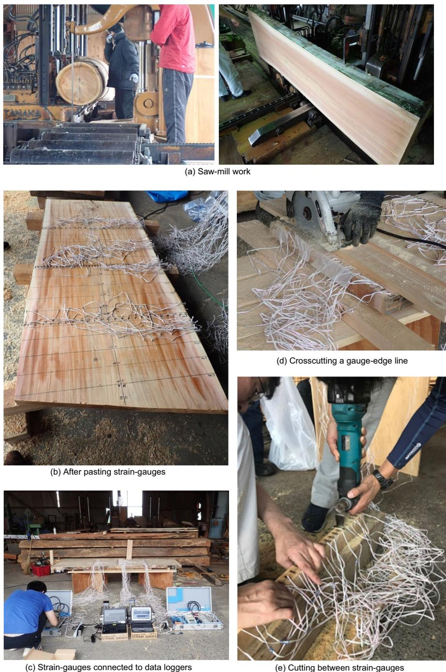
**Fig. 4** Sawing process of diametral planks and measurement of released strain
