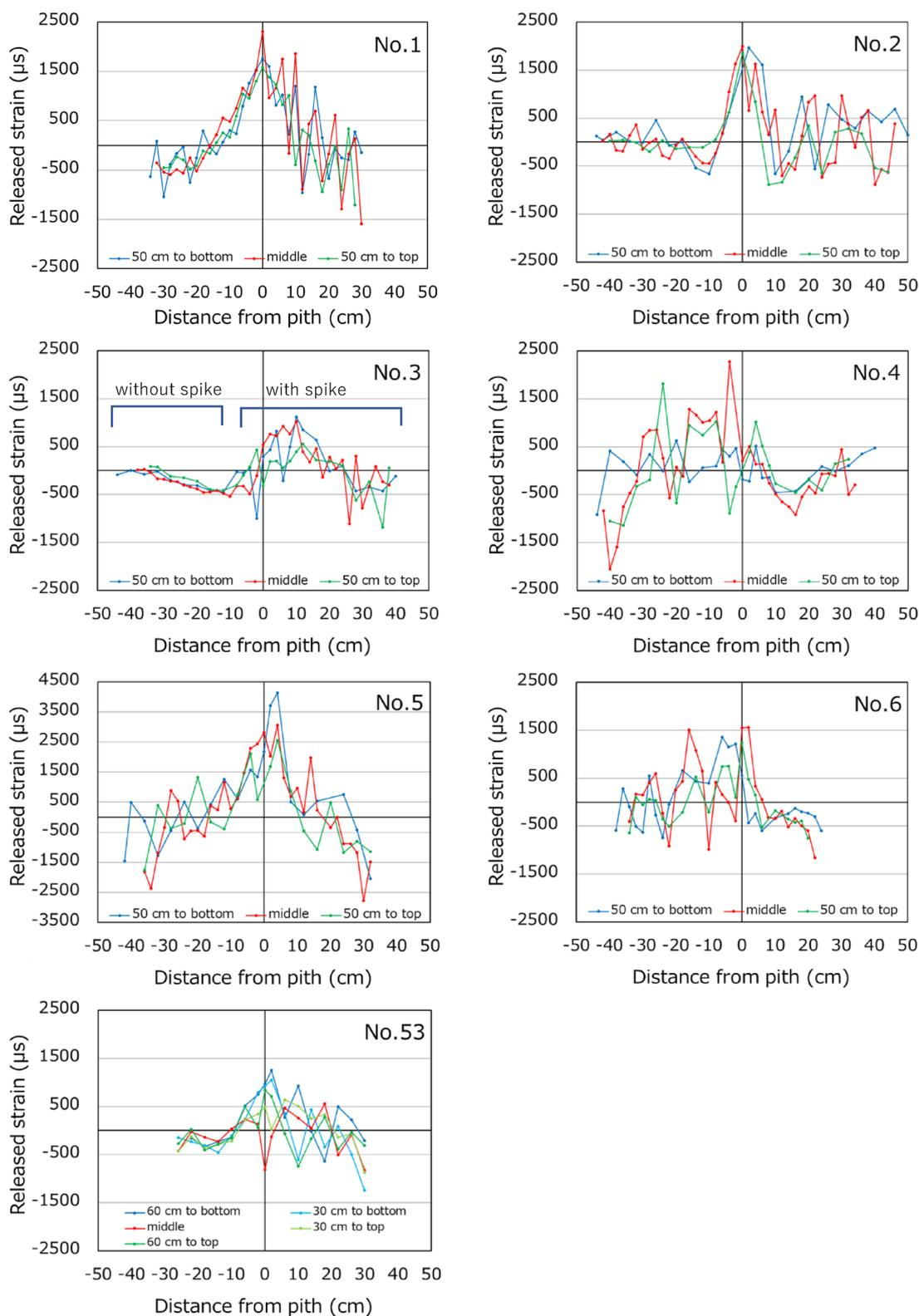
**Fig. 7** Released strain distribution among different longitudinal positions in the same log. For sample No. 3, radial ranges with/without spike-shaped strain are indicated
