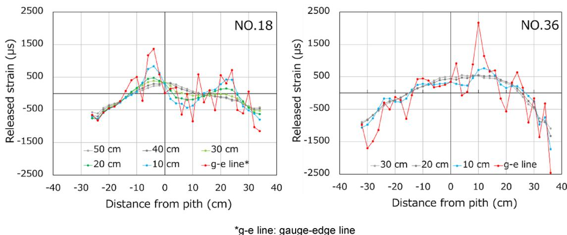
**Fig. 6** Typical examples showing longitudinal range of influence of spike-shaped stress. (Legends indicate the distance between the crosscutting position and the strain gauges.)
